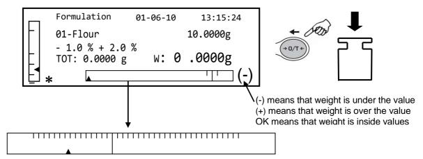
To facilitate the dosing operation, when the value of the component is approaching the threshold of the acceptable value, the dosing bar will automatically zoom.
