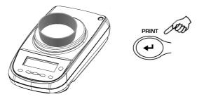
3. Load the number of pieces indicated on the display on the plate and press the **PRINT** button.
