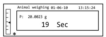
4. Once acquired, the weight will be shown on the display with an indication of the average weight detected.
