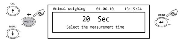
2. Set the desired time from 5 to 90 seonds using the **MENU** key to decrease and **CAL** to increase. Then confirm by pressing the **PRINT** button.
