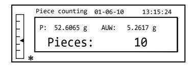
If the pieces to be counted have a weight that is too little with respect to the balance's resolution, an error message will be displayed.
