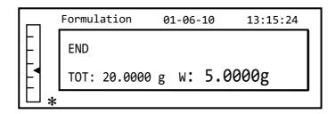
12. To exit from the screen and carry out a new formulation, press the **ON/OFF** button once. To exit from the program and return to the weighing screen, press the **ON/OFF** button two consecutive times.
