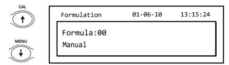
2. Choose the name of the formula (previously saved) using the **CAL** and **MENU** keys to scroll through the various formulas inserted.
