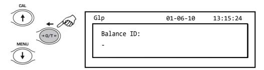
Enter the balance ID (it can be a series of numbers or letters, max 18 characters) using the MENU and CAL buttons to scroll through all of the available characters. To select uppercase or lowercase characters, press and hold the MENU button until the beeping stops.
