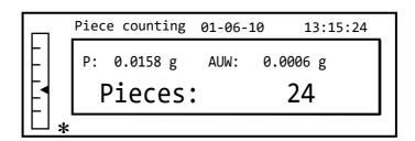
4. To exit from piece counting mode, press the **ON/OFF** button and the balance will return to the normal weighing conditions.
