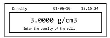
4. A different value can be entered by using the **CAL** and **MENU** buttons to increase and decrease the value, while pressing the **O/T** button to pass to the next value. During the entering phase, prolonged pressure on the **O/T** button allows you to delete the inserted value.
