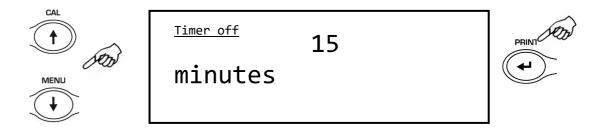
Select the desired auto-off modality. By pressing the MENU or CAL button it will be possible to scroll the various levels forward or backward; then confirm the choice with the PRINT button.
