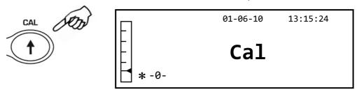
2. At the end of the calibration, the balance will return to normal weighing conditions.
