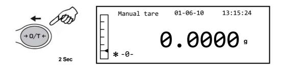
3. Now insert the desired tare value using the **CAL** and **MENU** buttons to increase and decrease the number, while pressing the **O/T** button to pass to the next number. During the entering phase, holding down the **O/T** button allows you to delete the inserted value.
