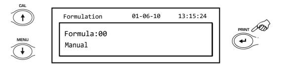
Select the number of the formula to save or modify using the CAL and MENU buttons to increase and decrease the value, after the word 'Formula'. Then press and keep pressed the PRINT button until the beeping stops to confirm the selection and enter the 'setup formula' menu.
