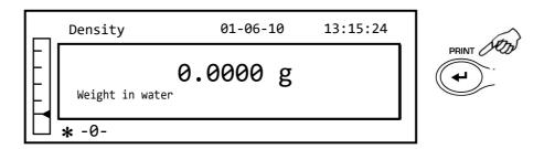
9. The result of the density calculation of the solid will now be displayed. If the balance is equipped with a printer, it will be possible to print the density value by pressing the **PRINT** button.
