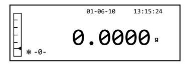
4. Put the objects to be weighed in the container. Read the value of the net weight on the display.
