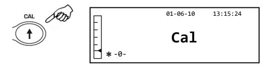
2. When the value of the calibration weight begins to flash, load the calibration weight on the plate.
