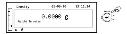
9. The result of the density calculation of the liquid will now be displayed. If the balance is equipped with a printer, it will be possible to print the density value by pressing the **PRINT** button.
