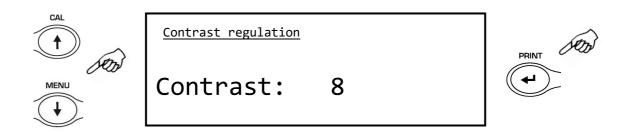
3. After having selected the desired contrast level, the screen relative to the balance parameters menu will be displayed again. It will now be possible to select another parameter or return to weighing mode by pressing the **ON/OFF** button.
